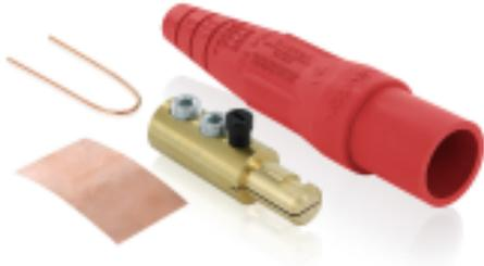
16 Series Taper Nose Cam-Type Male Plug, Contact & Insulator, Detachable, Double Set Screw Termination, 2/0 - 4/0 AWG, 400 Amp Max, Type 3R When Mated, Red
