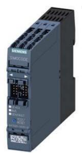
Basic unit SIMOCODE pro S, PROFIBUS DP interface 1.5 Mbit/s, 4I/2O freely parameterizable, Us: 110...240 V AC/DC, input for thermistor connection Monostable relay outputs, expandable by a multifunctional module
