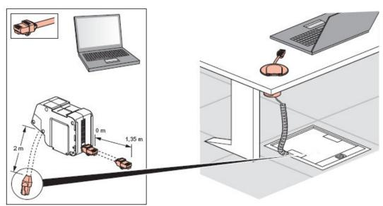
Installation with cellphone with retractable module USB/micro-USB
