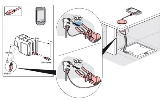
Installation with cellphone without retractable module USB/micro-USB  $\,$
